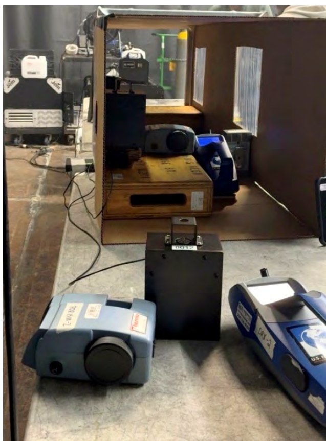
Figure 4. Closeup photo of testing setup of Set 2 instruments outside the tunnel exit (not all instruments shown in frame). This configuration was used for most foggers/hazers (excluding the low foggers).
