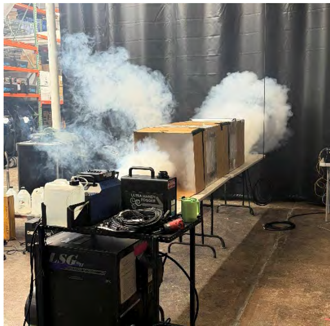
Figure 6. Example of fog stream into test tunnel during testing
