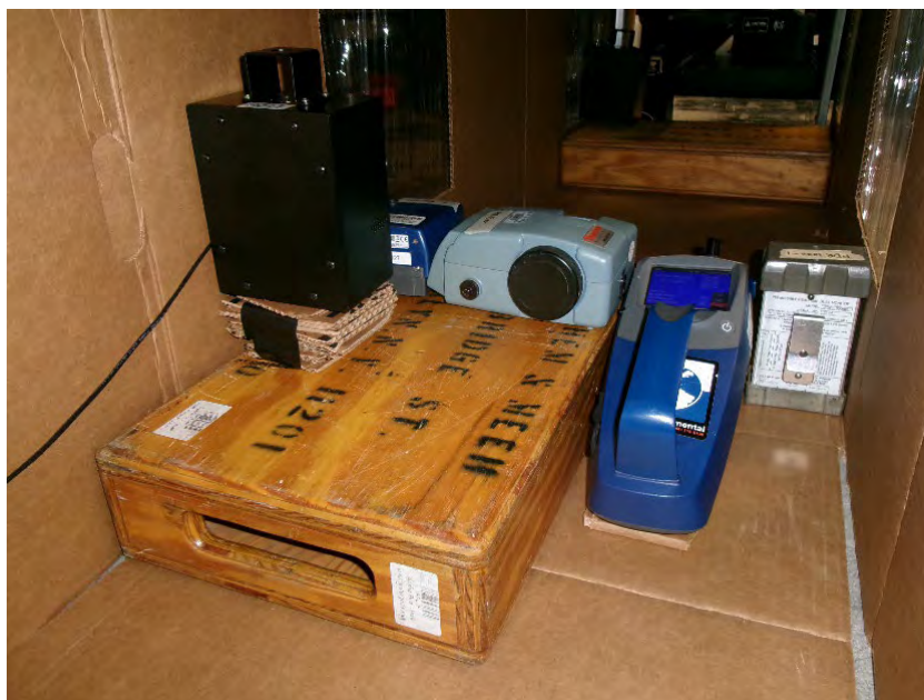
Figure 3. Closeup photo of testing setup of Set 1 instruments inside tunnel. This configuration was used for most foggers/hazers (excluding the low foggers).
