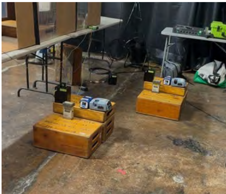
Figure 5. Setup of instruments for low fogger machine testing (Set 1 at front, Set 2 at rear)
